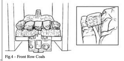
Place a single coal upon the two peaks of the coal matrix directly behind the centre line of the first row of coals. (see figure 5).
