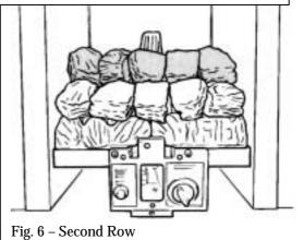
Place the remaining four coals behind the second row of coals, two each side of the centre coal shape formed within the matrix. (see figure 7).
